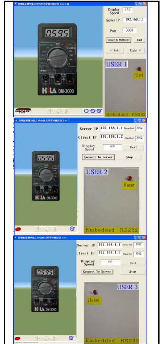
Figure 10 Diode measurement shown from the 3D virtual instruments of the members in the same group
