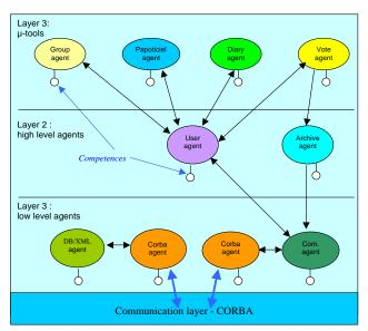
Fig. 12 Agent structure of Papoticiel on PLACID platform.
