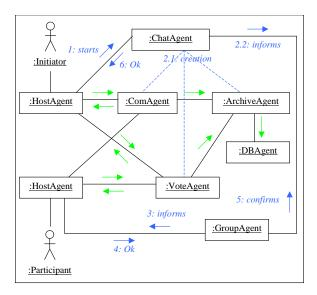
Fig. 11 Collaboration diagram illustrating scenario "begin-end".
