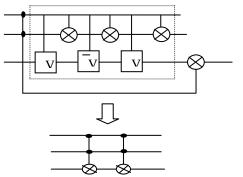
Fig 2: Fourth QHA section and its equivalent circuit
