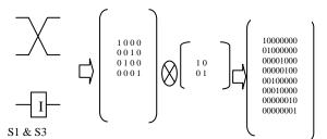
At this stage a swap gate is operated with a unitary identity gate and produces the state matrix.
