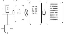
Here conjugate control square root of not gate is operated with unitary identity gate and produces the state matrix. In case of square root of not gate and conjugate control square root of not gate, in their gate matrix, we are using a 9 in place of i, which is a complex number. Whenever a multiplication operation between two 9 happens, we will just replace it by -1.
