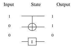
Here we are getting the output from this particular state input. It can be shown by operating the state matrix with the input.The equivalent decimal value of the input is represented by placing a 1 at that particular postion in the input matrix. The position of 1 in the output matrix below, represents the equivalent decimal value of the output of the state.
