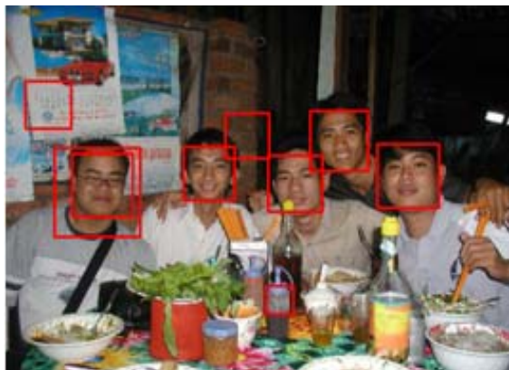
Figure 7: show the results of HSV method. It has about 3 errors on detecting faces and detects some none-faces objects as face.
