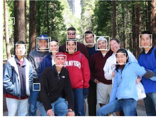
Figure 14: show the results of HSV method. It has 3 errors on detecting faces and detects some non-faces objects as face.
