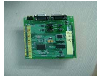
Fig. 9 Implemented MVB error detector
