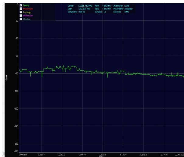
Figure 5: Power level in dBm versus frequency (2-2.2GHz)
