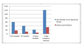
Fig. 9 comparison chart between OSI headers (TCP) with optional fields and optimized packet headers
