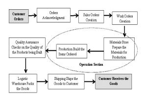
Fig. 1 Manufacturing Process Flow.
