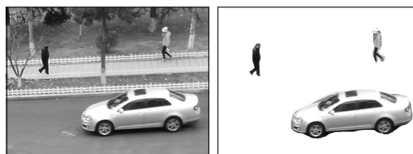
Fig 3. The background elimination effect for moving object after edge detection
