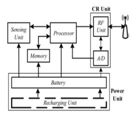
Fig.1 Hardware structure of a cognitive radio sensor node.
