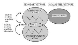
Fig.2 Proposed network architecture of cognitive sensor system.
