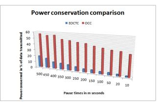
Fig 5: The Advantage of EOCTC over OCC in energy efficiency for data transmission
