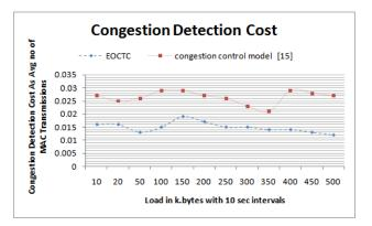
Fig 4: The advantage of EOCTC to minimize the cost to detect congestion over cross-layered congestion control model [15]
