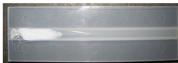
Fig. 4 Gas penetration result of 75% short-shot size
