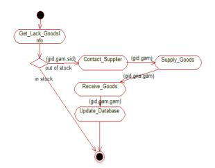
Fig. 2. an activity diagram of ordering system
