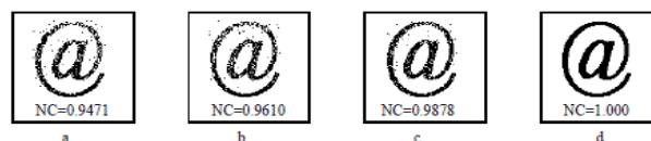
Fig 10: Extracted watermarks under Gaussian noise, (a) generations = 25, (b) generations = 50, (c) generations = 100, (d) generations = 150
