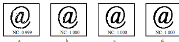
Fig 11: Extracted watermarks under JPEG attack from different host images using 100 generations, (a) Lena image, (b) Fruit image, (c) Baboon image, (d) Boat image
