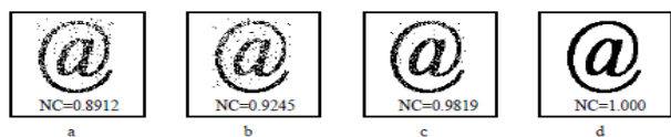
Fig 6: Extracted watermarks from the girl image: a) Low pass filter b) Median filter c) Gaussian noise d) JPEG compression
