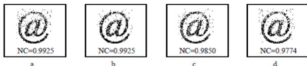
Fig 8: Extracted watermarks under Gaussian attack: a) 5% Gaussian noise added b) 4% Gaussian noise added c) 3% Gaussian noise added d) 1% Gaussian noise added
