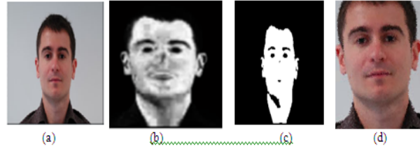
Fig 11 (a) input image, (b) detected skin Region (c) binary image after skin region detection, (d) Cropped output face
