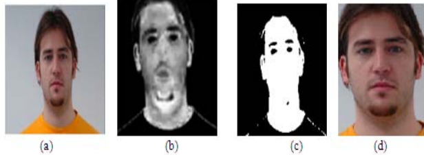
Fig 12 (a) input image, (b) detected skin Region, (c) binary image after skin region detection, (d) Cropped output face
