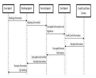
Fig 3. Sequence diagram of e-transaction related messages
