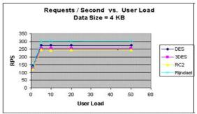
Fig 8. Request per second Vs User Load
