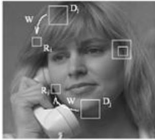
Fig. 2 The transform between domain block ( D_i ) and range block ( R_j ).
