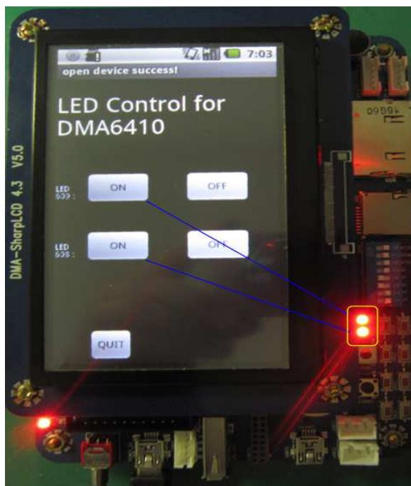
Fig. 12 (a) The experimental result of all LEDs on
