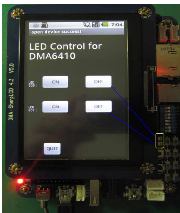
Fig. 12 (b) The experimental result of all LEDs off
