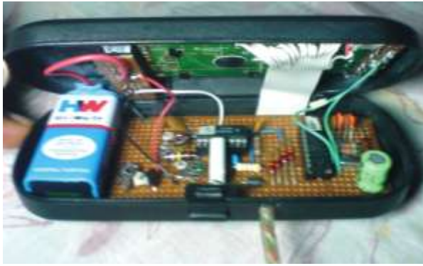
Fig. 7: Case opened showing assembled circuit on matrix board.
