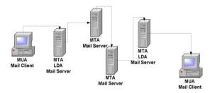
Fig. 1 The flow of the message through the various mail components. Source [14]
