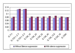
Fig.6 Packet End to End Delay with silence suppression (sec)
