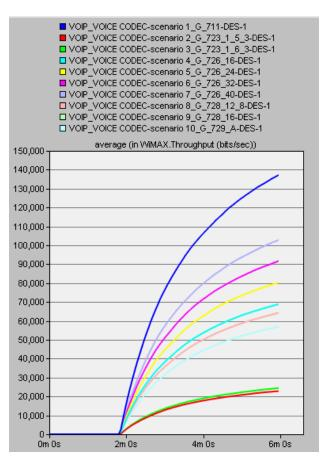
Fig.5 Relative Throughput of voice codecs (bits per sec)
