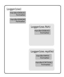
Fig. 2 Logger Hierarchal Structure
