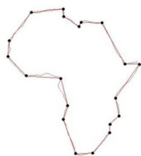
Fig 20: the dominant points in map's boundary after algorithm operation and removing the dominant points with AEV < 10 .
