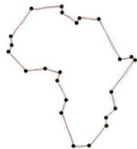
Fig 19: the dominant points in map's boundary after algorithm operation and removing the dominant points with AEV < 2 .
