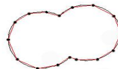
Fig 16: picture of a tab after algorithm operation and removing the dominant points with AEV<10.
