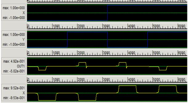
Fig.7 Simulated waveforms for Feynman gate circuit.
