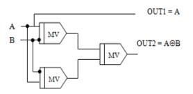
Fig. 5 Block Diagram of QCA is the Feynman gate.
