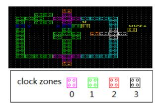
Fig. 6 Design QCA is the Feynman gate.
