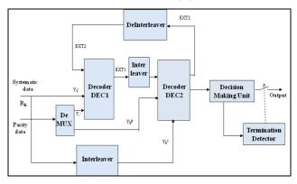
Figure 1: The structure of Turbo Decoder.
