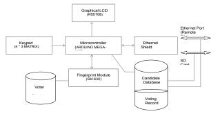
Figure 1: Block Diagram of Proposed Secure E-Voting System
