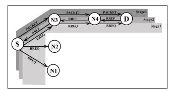
Fig.1 Ad-hoc On-demand Distance Vector routing algorithm
