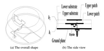
Fig. 1 proposed circular patch Antenna.
