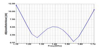
Fig. 3 Axial ratio of the antenna.
