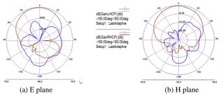
Fig. 4 Simulated Circularly Polarized Radiation Patterns at 1575MHz.
