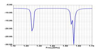
Fig. 2 Return loss of the proposed antenna.
