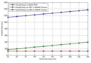
Fig. 7 Impact of Router Discovery on Handoff delay
