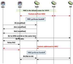
Fig. 5 Timing diagram for the proposed scheme
