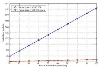
Fig. 9 Packet Loss as a function of packet arrival rate
