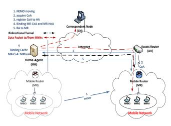
Fig. 1 NEMO BSP operation where numbers represent sequenced operation for NEMO
