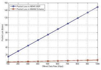
Fig. 8 Packet Loss as a function of offered data rate
