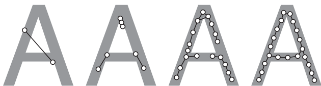
Fig.2 Different steps of convergence of the network for the character "A". These figures show the networks after 0, 4000, 12000, and 80000 steps (from left to right). At the end of the adaptation process the connection between the nodes represents the structure of "A".
