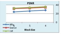
Fig. 6: The effect of block size on the PSNR
