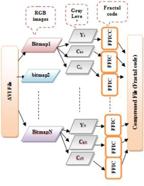
Fig. 1: Encoding flowchart of AVI file (Compression)
