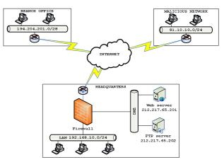
Fig. 8 Example of company network secured by a firewall
