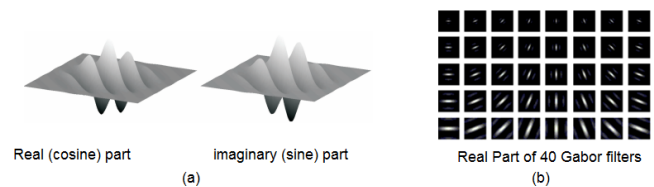
Fig. 4- (a) Gabor filters Real and Imaginary parts-(b) 40 Gabor filters of 5 frequencies and 8 orientations
