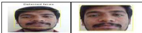
Fig. 2: Frontal face detection using Face detector object
