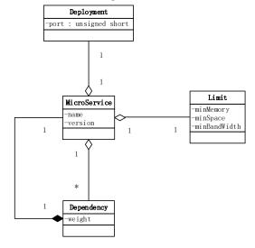
Fig. 3 micro-service deployment description model
