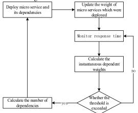
Fig. 5 update process of the dependent weight
