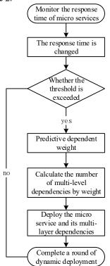
Fig. 2 flow chart of micro service dynamic deployment
