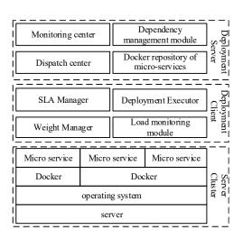
Fig. 1 Dynamic deployment architecture
