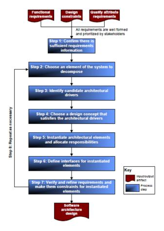
Fig. 1 Software architecture design process.
