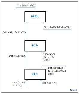
Fig. 5 Congestion control scheme in node *i*
