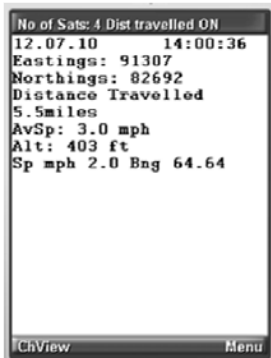
Fig. 6 A view showing the British National Grid reference system
