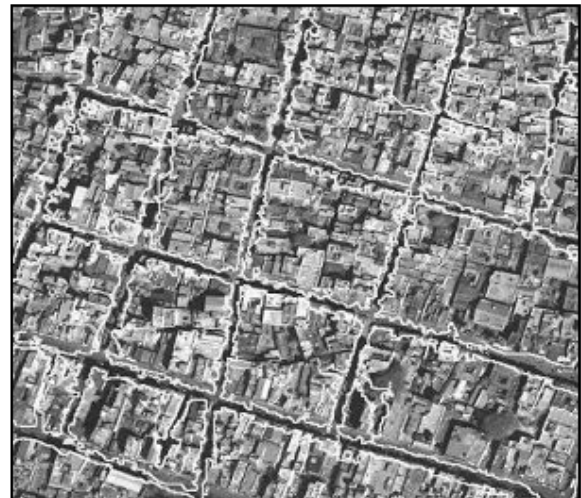
Figure 4. Extracted road network using Mean Shift Method
