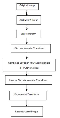
Fig. 1. Overview of the proposed method (Combined Bayesian MAP Estimator and ST-PCNN) The noisy ultrasound image is given as H(k, 1) = i(k, 1)\*J(k, 1) + f(k, 1) (1)
