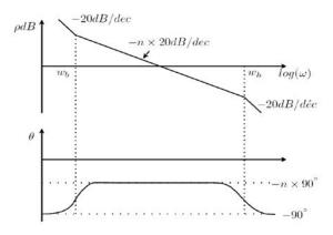
Fig. 1. Bode diagram of the fractional integrator
