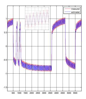
Fig.13. Measured and estimated currents with fractional model  $H_{n_1,n_2}$
