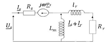
Fig.3. Conventional equivalent diagram of Park's model
