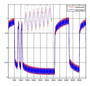
Fig. 11. Measured and estimated currents with fractional model  $H_n(s)$
