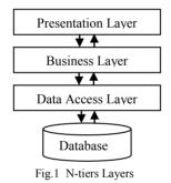
Each Layer can be developed independently of the other provided that it adheres to the standards and communicates with the other layers.
