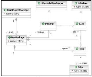
Fig. 4 Simplified meta-model of DaoPackage
