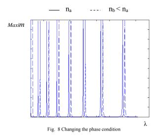
By changing the index of the optical wave guide, we change the distribution of the maxima in the core-Perot (Fig. 8), since it creates an additional phase shift.
