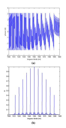
Fig. 6 (a) Phase (rad) in a sampled grating (b) Reflectivity (amplitude) in a sampled grating
