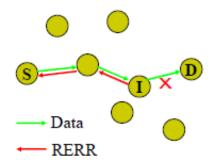
Fig 6 AODV routing protocol with RERR message
