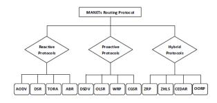
Fig.4 Different type of routing protocols in wireless Ad-hoc network
