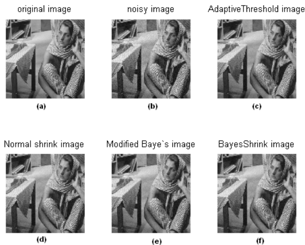
Fig. 5: Quality performance of different denoising methods for Barbara image (noise standard deviation \sigma_V = 0.001 ) (a) Original image (b) Noisy Image (PSNR=69.07) (c) Adaptive Threshold (PSNR=73.01) (d) Normal shrink (PSNR=73.15) (e) Modified Baye's shrink (PSNR=73.05) (f) Baye's Shrink (PSNR=73.02)
