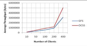
Figure 5: average throughput: during write operation
