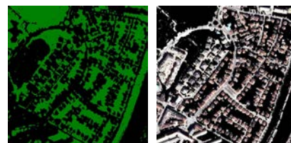
Fig. 3 (a) Trees and forest segmentations from NDVI index. (b)Detection of houses and street.
