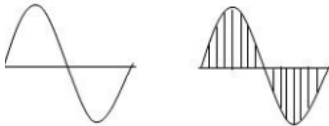
Fig. 3 Sampling of the Sine Wave followed by Quantization process.
