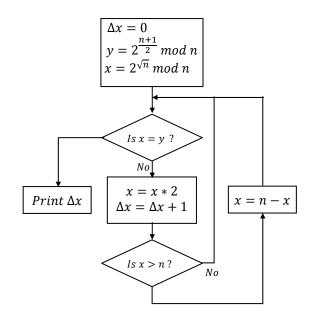
Fig. 5: One sample flow diagram to finding  $\Delta x$
