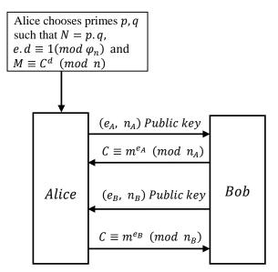
Fig. 1: Diagram of RSA Encryption and Decryption
