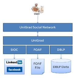
Fig. 6 The Application Architecture
